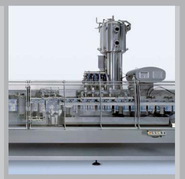
A bag forming, filling and sealing machine works at high speeds. It has stroke lengths of 1500 to 2100 mm, the average service performance is 30000 kilometers a year. The Franke Dynamic Aluminium Roller Guide used must be resistant to the aggressive environmental conditions, such as salt, sugar and splash water.
