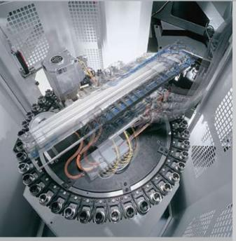
In tool changers at machining centres, our bearing assemblies help to ensure that different tools are fed quickly and precisely into the machining head.
