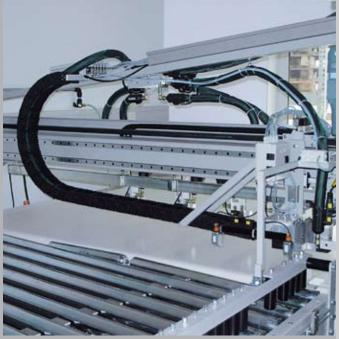
The Franke Dynamic Aluminium Roller Guide is also used on packaging machinery for mattresses. In addition to cleanliness, the mobile function of the guide unit must be ensured, to avoid soiling the mattresses.
