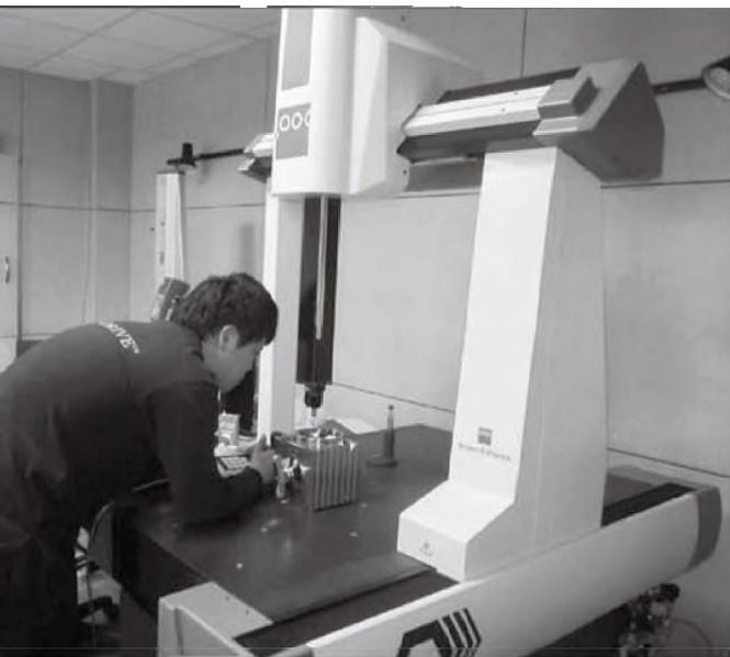
Pre--inspection:All raw materials are certified that ingredients are correct by suppliers and QC dept. before process procedures. Each part has to be measured strictly by gauge · caliper or CMM in order to ensuring the dimensions are with in tolerance range according to the corresponding drawing.
