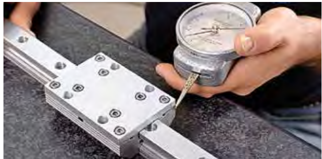
Diagram 2: Measure slide resistance
