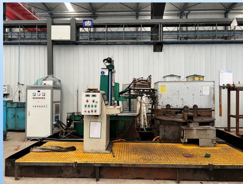
2m gear teeth quenching lather ( heat treatment process)
