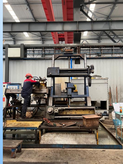
2m slewing bearing raceway quenching lather ( heat treatment process)
