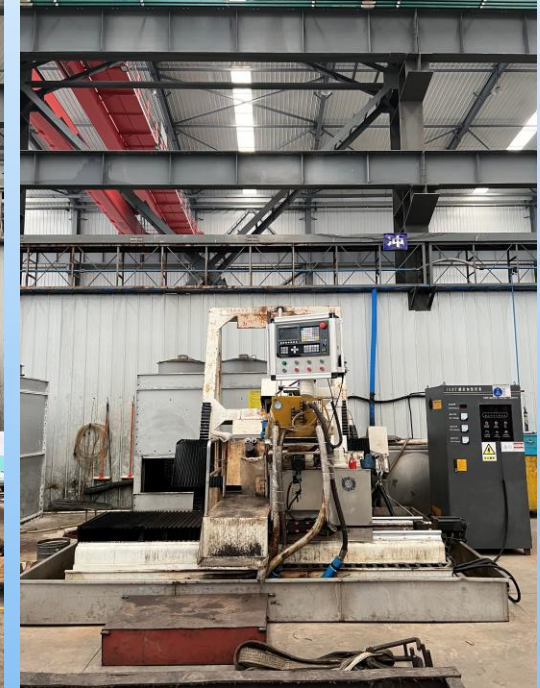
1.7m slewing bearing raceway quenching lather ( heat treatment process)
