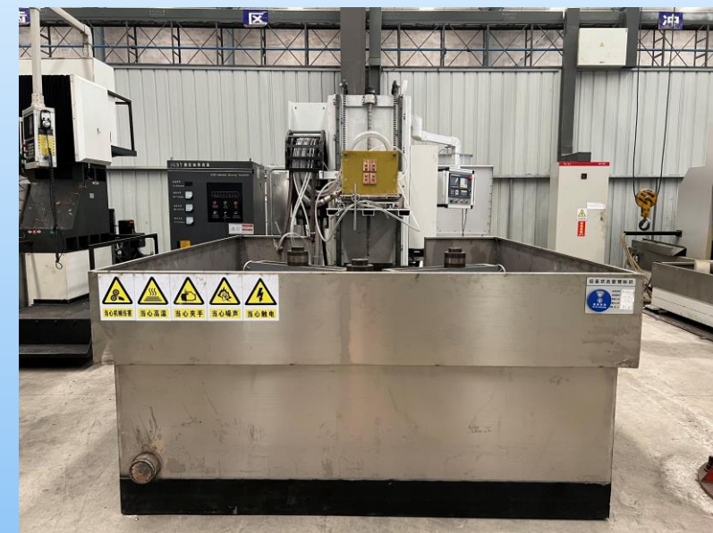
2.5m gear teeth quenching lather ( heat treatment process)
