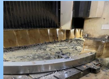
Mounting Holes Drilling
