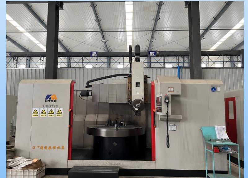
1.7m raceway high precision CNC machine
